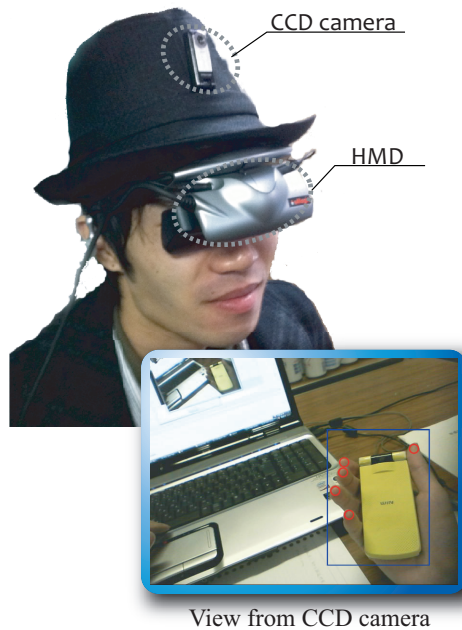
Fig. 8 HMD and camera in our testbed AR tool.
