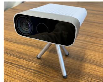
図 6: Azure Kinect DK
